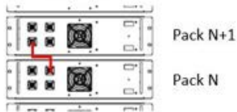
Wrong connection mode 2
